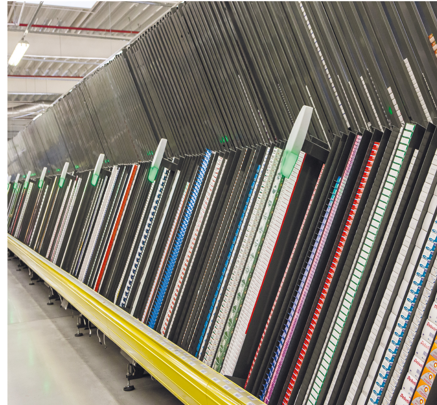
An automated order picking machine handling pharmacy orders at a PGF warehouse
